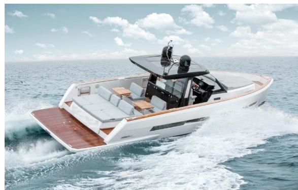
With a total length just 80 cm longer and 25cm beamier than the Fjord 40', the Fjord 44 open offers a series of significant changes. Starting with the extra large hydraulic bathing platform which enables you to carry a Williams MiniJet or a Seadoo Spark weighing up to 300Kgs. The stairs which are built into the platform unfold to offer comfortable steps communicating the submerged platform with the main deck. Another major feature of the boat is the Sunbed which is separate from the seating.
